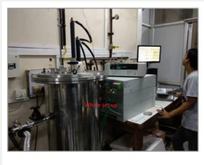
The figure above shows the fully integrated smart superconducting fault current limiter in operation.
